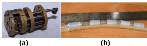
Fig. 6 (a) A driving segment and (b) Microrobot as a whole [7].
