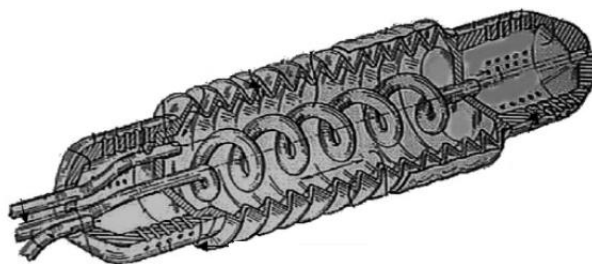
Fig. 14 Pneumatic lay-out of the microrobot: (a) cylindrical clamber with suction holes and hemispherical tips; (b) rubber bellow; (c) service pipes [15].
